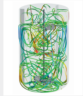
CFD simulation - Flow pattern in a fermenter
