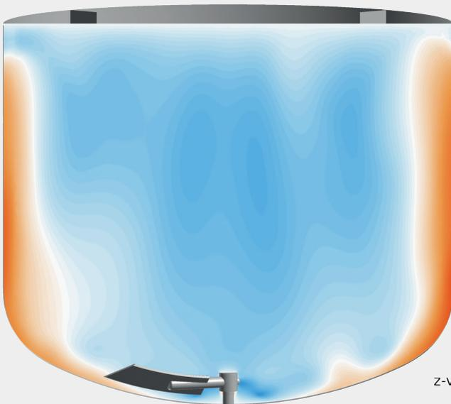
Comparison of the axial flow velocities induced by the ENDSFOIL
