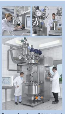
Customers have the possibility to test and optimize their processes on all SOLIDMIX unit types in the EKATO SYSTEMS test facility.
