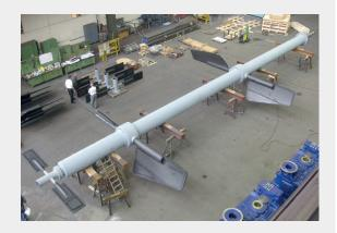
Agitator for a 6,500 m³ storage tank
