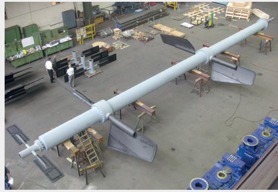
Agitator for a 6,500 m<sup>3</sup> storage tank
