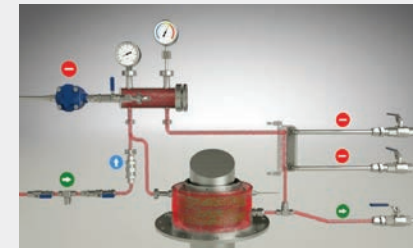
Step 1: Flow-through sterilization Cleaning and sterilizing all parts with fresh steam during standstill of the agitator
