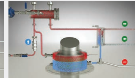
Step 2: System-filling Filling the system with sterile condensate during standstill of the agitator
