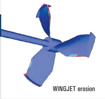
Comparison of areas exposed to wear on blade tips
